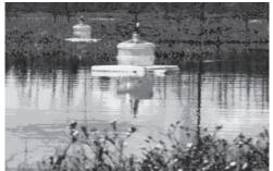
A static floating chamber measuring the rate of buildup of  $CO_2$  and  $CH_4$  gases over time inside the chamber
